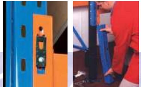
**Storax SP80** offers the full range of frame protection, from the column guards and upright protectors that are used in 'normal' environments, through to sacrificial legs, where high incidence of fork truck impact is expected.
